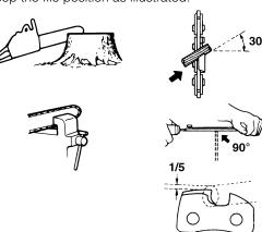
After each cutter has been filed, check the depth gauge and file it to the proper level as illustrated.
